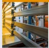
Our in-house powder coating facility offers finishing in a variety of colours with RAL, BS or colour matched powders. CAPALEX is able to coat in both aluminium and steel components in lengths from a few millimetres to 6 metre lengths.
